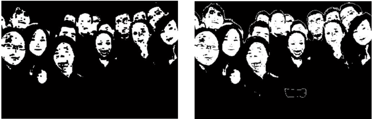
Figure 5.2: MATLAB implementation :Result after thresholding and Connected Component Labeling
